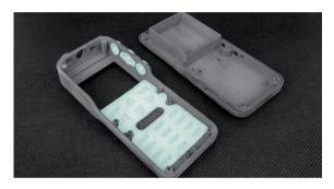
Maciej Burzyński from Sybet prototyped with Sinterit Lisa a portable handheld receiver for KGHM, the world leader in copper and silver production. Printing the whole set of radiotelephone parts with PA12 and Flexa Grey costs less than 600 USD and takes about four days.
