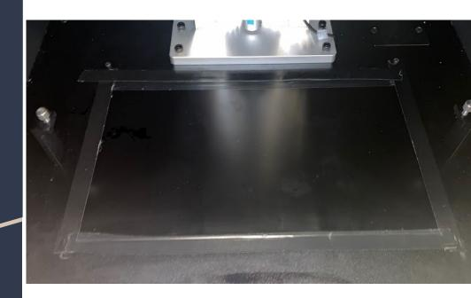
Check to ensure the build plate is level to the LCD screen.
