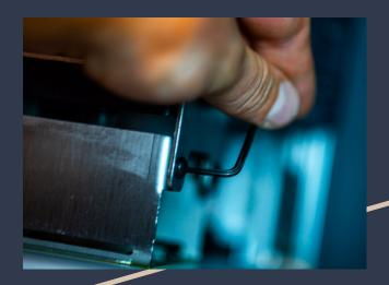
Recheck again to make sure the paper does not slide under the plate. GENTLY press down the plate to make sure it is level to the LCD and carefully re-tighten the bolts, again double checking to make sure the paper does not slide between the plate and LCD.
