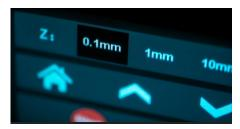
Once the plate is level to the screen, press the back button and then press the button that says Set Z=0 This will store the new height as the default Z axis as 0 with the new height.
