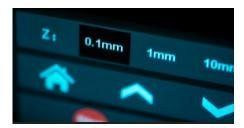
Once the plate is level to the screen, press the back button and then press the button that says Set Z=0 This will store the new height as the default Z axis as 0 with the new height.
