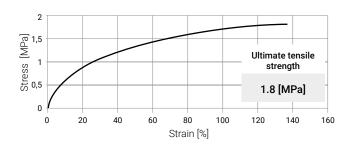
While the tensile stress does not exceed 0.8 [MPa], after load release, the test specimens retain their shape, with no external damage observed (e.g. fractures). The test specimens fracture when a max tensile stress of 1.8 [MPa] is applied.
