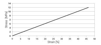
While the compressive stress does not exceed 12 [MPa], after load release, the test specimens retain their shape, with no external damage observed (e.g. fractures).
