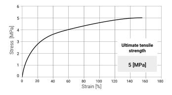
While the tensile stress does not exceed 2.3 [MPa], after load release, the test specimens retain their shape, with no external damage observed (e.g. fractures). The test specimens fracture when a max tensile stress of 5 [MPa] is applied.
