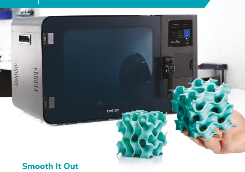
Zortrax Apoller is a smart vapor smoothing device that automatically removes visible layering from FDM 3D prints. It works in three simple steps. First, the model has to be placed inside the smoothing chamber. Second, the door has to be closed and settings chosen with an intuitive touch interface. Third, the model has to be taken out of the chamber once the smoothing process is done. Vapor smoothing performed in Zortrax Apoller does not affect the model's details nor dimensional accuracy.
