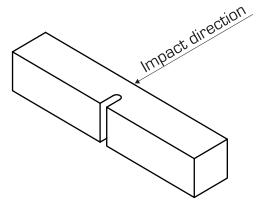
Picture 2. Notched beam used for the Charpy Impact Test
